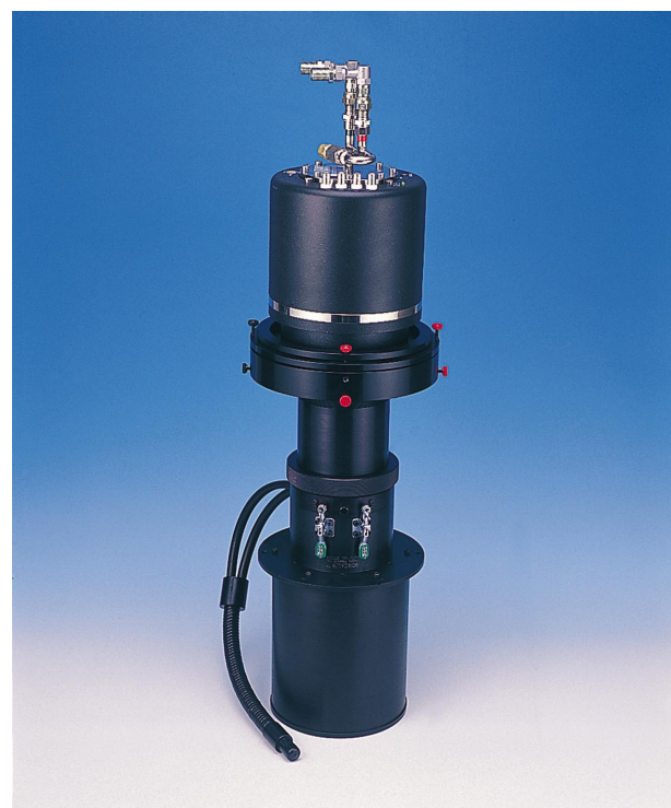
Figure 1. The area-imaging components of the LEADseeker (APBiotech, Amersham, UK), including a large telecentric lens and a cooled charge-coupled device (CCD) camera (mounted above the lens). The lens incorporates an epi-illumination mechanism, fed by a fibre-optic 'tail'.
